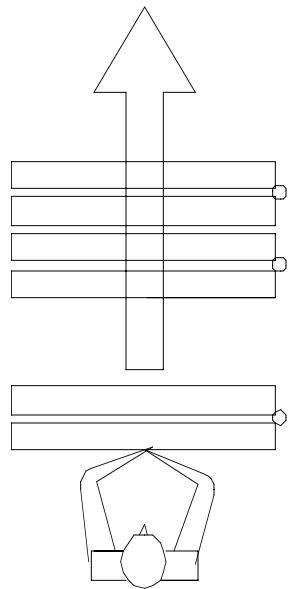
6. Slightly separate the next pair. Keep panel pair in extended flat position until near the stack. Fold by pushing on hinge. Repeat Step 5.
