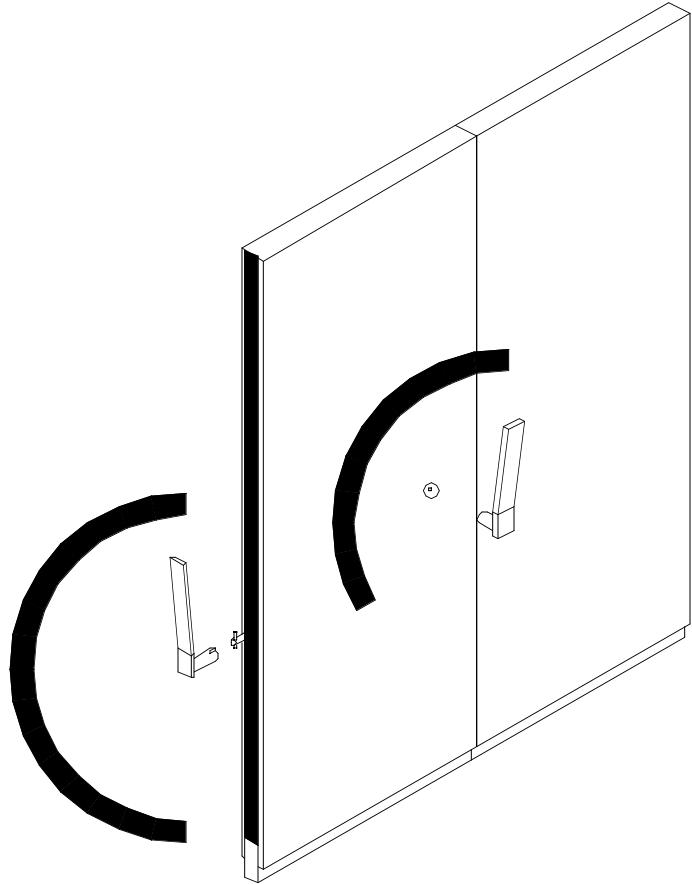
10. Put operating handle into panel face cup and rotate until there is a pronounced cam action.
